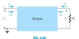
Determining the current gain using the voltage gain.
