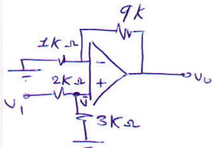
$$V_{o1} = (1 + \frac{9k}{1k}) \bar{V} = (10) \frac{3V_1}{5}$$
