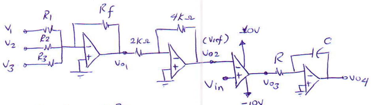
$$R_1 = R_2 = R_3 = 0.2 R_f$$
