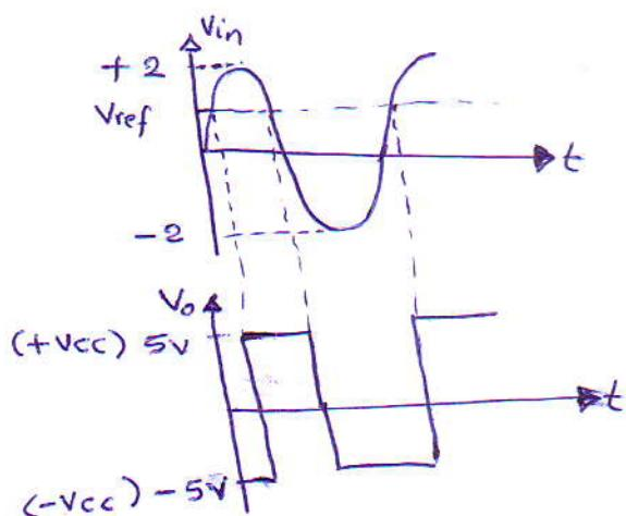
H.W: If  $V_{ref} = 0$  for the circuit above; find  $V_o$  waveform.
