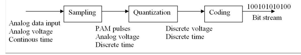
**Sampling:** The input analog data signal is sampled at twice the highest significant frequency of the data signal. Each sample represents a narrow pulse whose amplitude is proportional to the value of the original data signal. This process is known as Pulse Amplitude Modulation (PAM).
