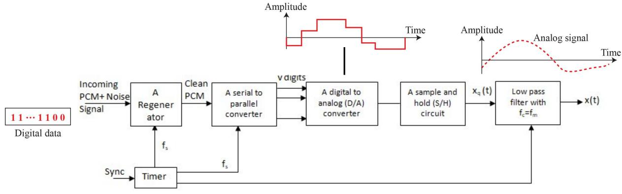
To recover an analog signal from a digitized signal, following steps are needed:
