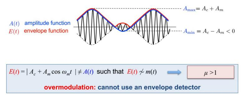
When  $A_c < A_m$  hence  $\mu > 1$  (overmodulation). In this case, the option of envelope detection is no longer viable. We then need to use synchronous demodulation. Note that synchronous demodulation can be used for any value of  $\mu$ . The envelope detector, which is considerably simpler and less expensive than the synchronous detector, can be used only for  $\mu < 1$
