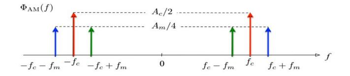
**Example:** Sketch  $\phi_{AM}(t)$  for modulation indices of  $\mu = 0.5$  and  $\mu = 1$ , when  $m(t) = B \cos \omega_m t$ . Solution:
