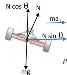
$$\left(\begin{array}{c} \rightarrow \\ + \end{array}\right) \quad \sum F_n = ma_n; \quad N \sin \theta = m \frac{v^2}{\rho} \quad (1)$$
